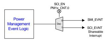
Figure 4-12 Power Management Events to SMI/SCI Control Logic
