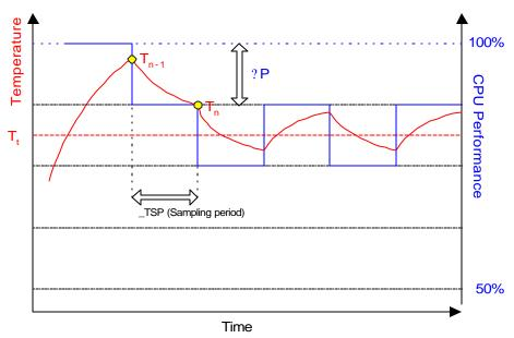
Figure 12-2 Temperature and CPU Performance Versus Time
