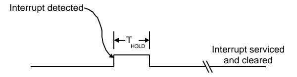
Figure 13-3 EC Interrupt Waveform
