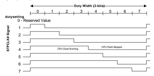
Figure 4-15 Example Control for the STPCLK#
