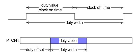
Figure 4-14 Throttling Example
