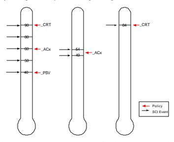
Figure 3-10 Example Thermal Cooling Implementations
