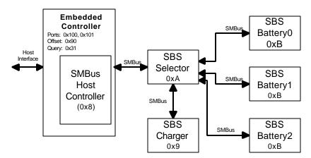
Figure 11-3 Smart Battery Subsystem
