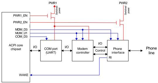
Figure 3-2 Example Modem and COM Port Hardware
