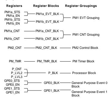
Figure 4-6 Register Blocks versus Register Groupings
