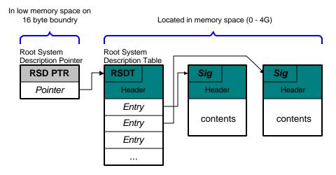
Figure 5-1 Root System Description Pointer and Table
