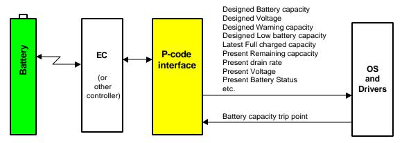
Figure 3-3 Control Method Battery Diagram
