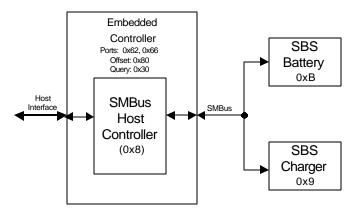
Figure 11-2 Single Smart Battery Subsystem
